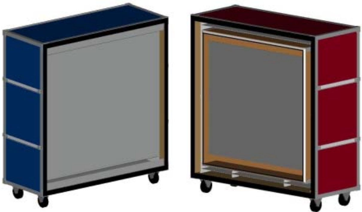
Figure 4. View at the Open Universal Guarded Hot Box
