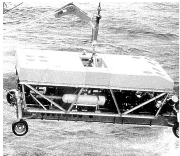
Figure 9 Nexans’ CapJet cable-burying ROV being lowered into the water
