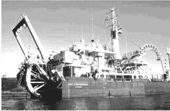
Figure 7: Skagerrak laying vessel (Nexans)
