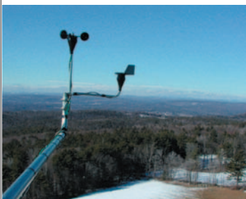
Anemometer & vane in the field.
